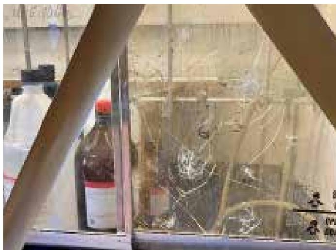
mantle which was set to slightly below the “low” setting. The researcher left the fume hood and went to an adjacent room to work. While working in the adjacent room, the researcher heard a loud explosion in the room where the tosyl azide experiment was being heated. When the researcher went into the room where the explosion occurred, there was a lot of smoke and fumes, but no observable fire.
