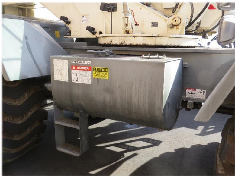
Map ID: 8 Designation: TEREX Crane Oil Type: Hydraulic oil Size: 80 gallons Containment: Double-walled tank Location: Outside Building 2 on Wharf
